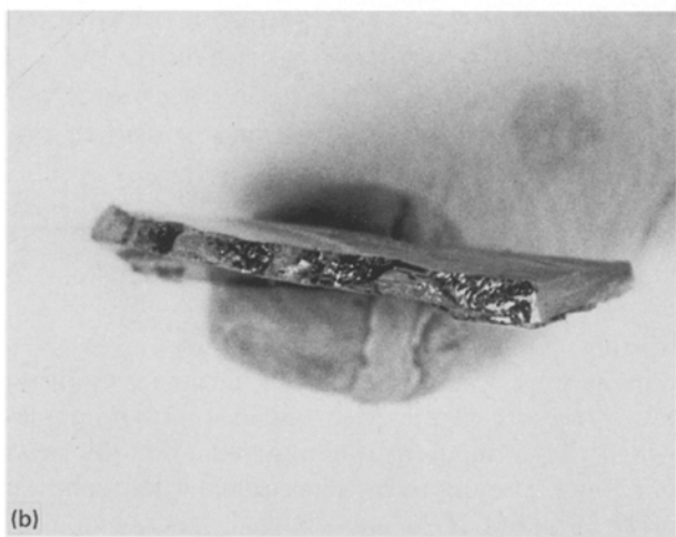
Figure 1 Photographs of grown SnSe 2 crystals: (a) view perpendicular to the layers, and (b) parallel to the layers.
